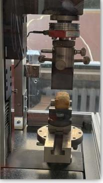
Texture Profile Analysis -Three-point bending test
