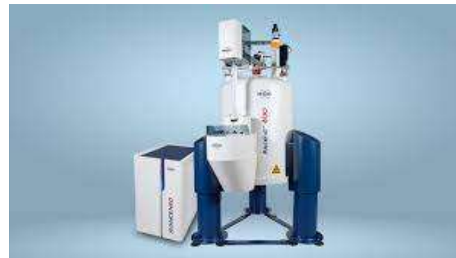
NMR spectrometer Monodimensional and NOESY experiments with suppression of main signals
